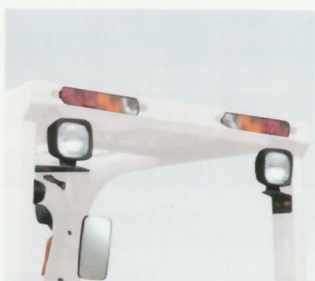
Rear working light
